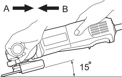
ALWAYS hold the tool firmly with one hand on housing and the other on the side handle. Turn the tool on and then apply the wheel or disc to the workpiece.
