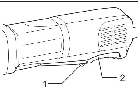
► 1. Lock-off lever 2. Switch lever
