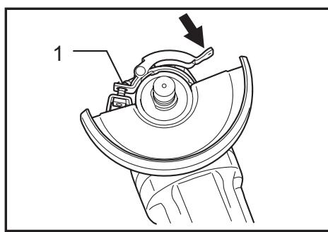
Pull the lever in the direction of the arrow after loosening the screw. Mount the wheel guard with the protrusion on the wheel guard band aligned with the notch on the bearing box. Then rotate the wheel guard around 180°. Fasten it with the screw after pulling lever in the direction of the arrow for the working purpose. The setting angle of the wheel guard can be adjusted with the lever.
