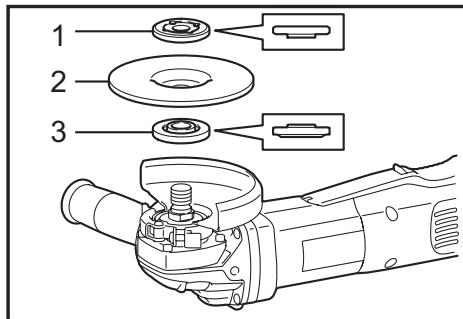
To tighten the lock nut, press the shaft lock firmly so that the spindle cannot revolve, then use the lock nut wrench and securely tighten clockwise. To remove the wheel, follow the installation procedure in reverse.
